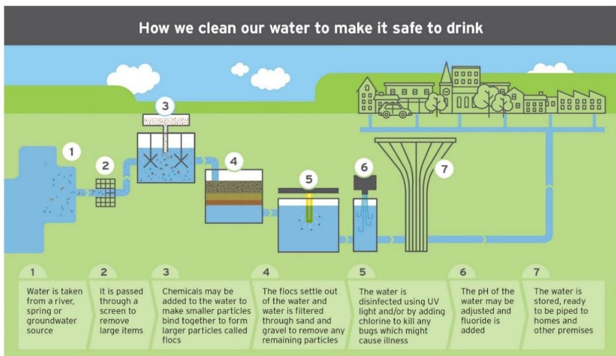
Figure 6: Steps in the drinking water supply process
