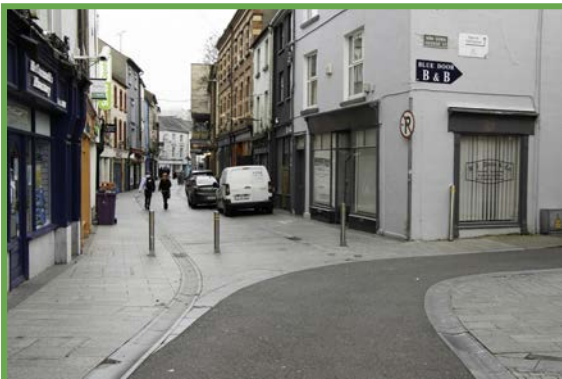
Main Street, Wexford: These hydraulic bollards are lowered into the ground when delivery or emergency vehicles need to use the laneway. This maintains safety for pedestrians without hindering necessary traffic.
