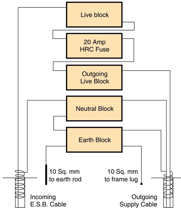
**FIGURE 5.3: INTERNAL ELECTRICAL ARRANGEMENT
