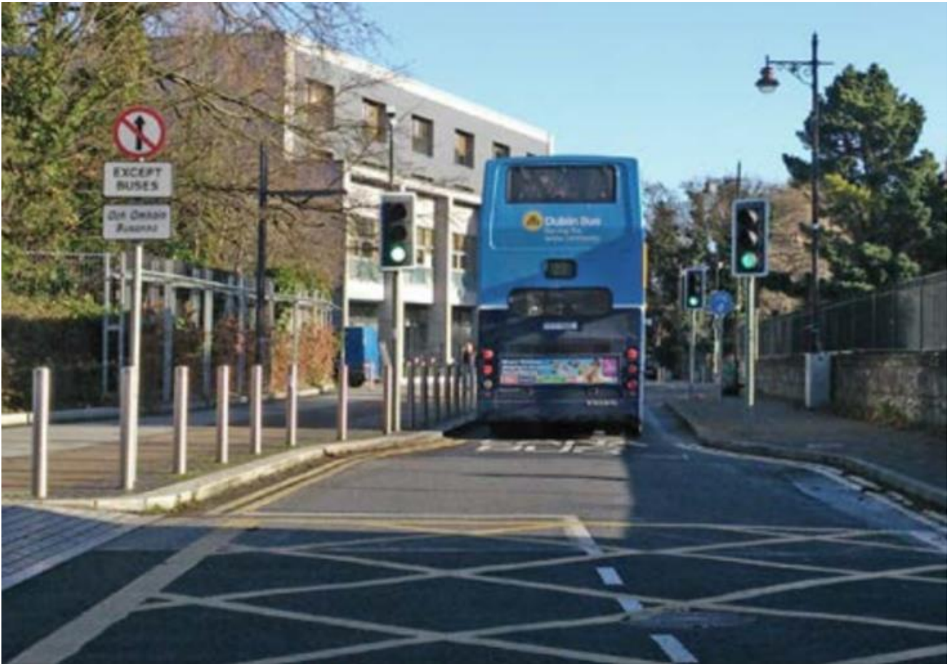
Figure 6-2: Bus Gate in Tallaght, Dublin. Source: P.56, DMURS, 2019, DTTaS.
