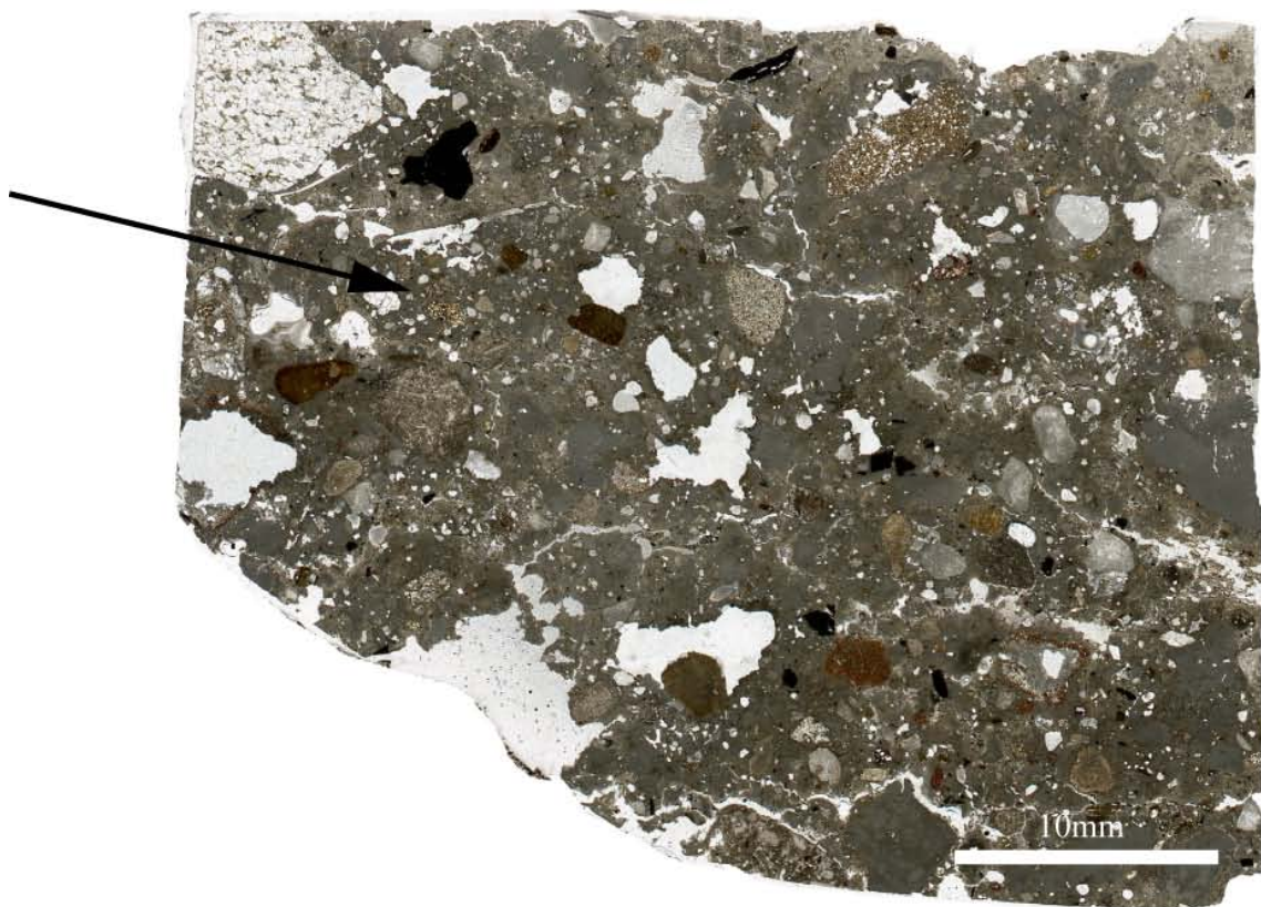
Figure 2. Scanned image of Sample B, Evan's home, Kilkenny, showing gravel and coarse sand grade in fine-grained binder. Area illustrated in Figure 4 is arrowed.
