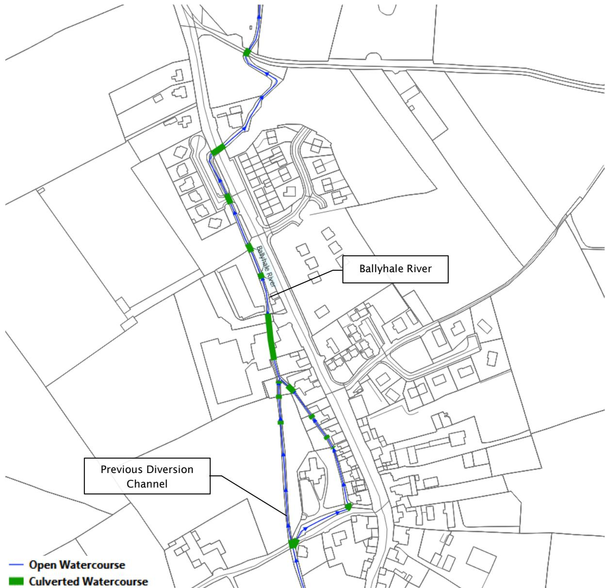
**Figure 2-2 Ballyhale River Structures**
