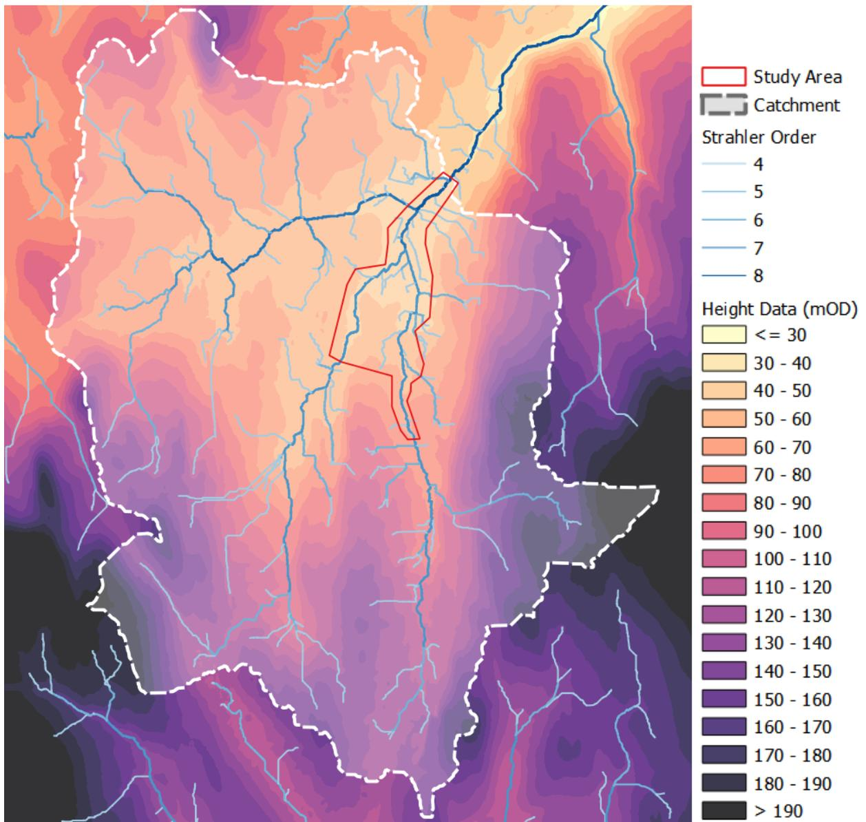
**Figure 4-1 Topographic Data and Flow Accumulation Analysis**
