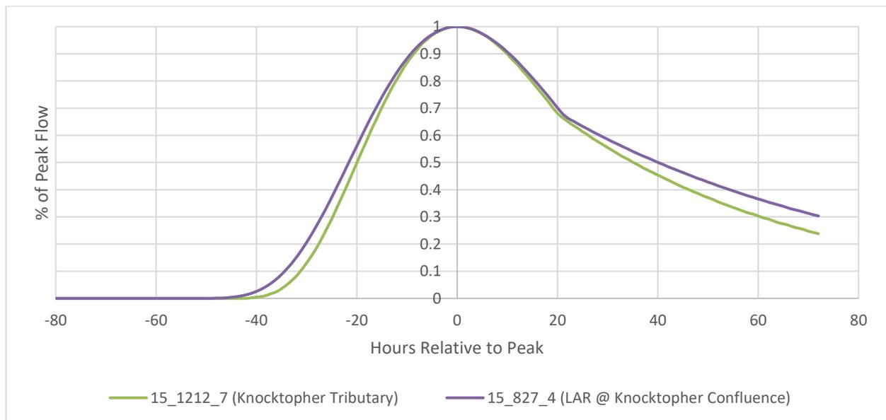
**Figure 9-2 Design Hydrograph Shapes**
