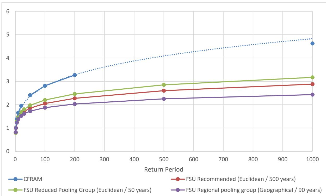
**Figure 8-1 CFRAM - FSU Growth Curve Comparison (HEP 15\_1358\_3, Pivotal Station: 15001 Annamult, Distribution: GLO)**
