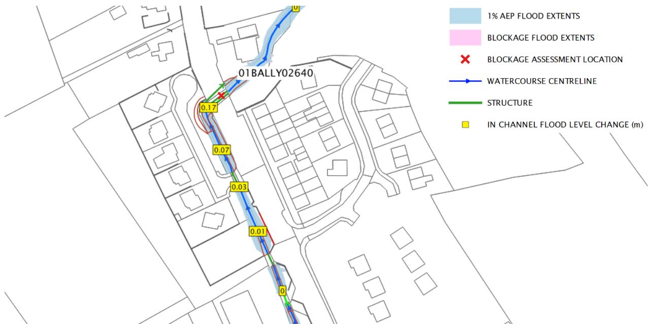
**Figure 7-9 Proposed Scheme – 01BALLY02640 - 50% Blockage**
