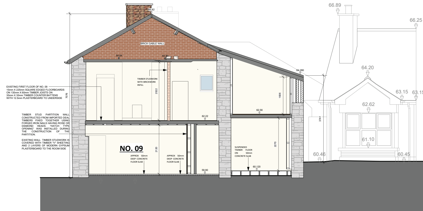
04 EXISTING SECTION THROUGH NO. 09 092 1:50 @ A1
